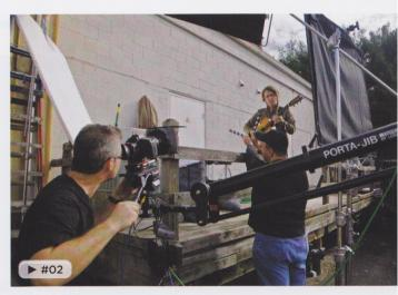
▲ The camera is attached to a jib arm to give it fluid movement. The Director of Photography can literally "float" the camera through the scene.
