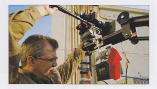
**Pedestal (Boom):** A pedestal move describes moving a camera up and down in physical space. It is different from a tilt in that the camera's physical axis is changing. Pedestal moves typically require advanced camera support like a boom or crane to lift the camera. Pedestal shots are often combined with other moves like pans and tilts to add drama to a shot.
