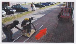
**Dolly:** A dolly is both a device and a movement type. The camera is mounted on a wheeled cart or platform. It then can move in and out (essentially closer or further) to the subject. The use of a dolly can create a very dramatic shot that engages the viewer. The use of a dolly generally requires an operator (called a dolly grip) to physically push the cart and control the speed of movement.
